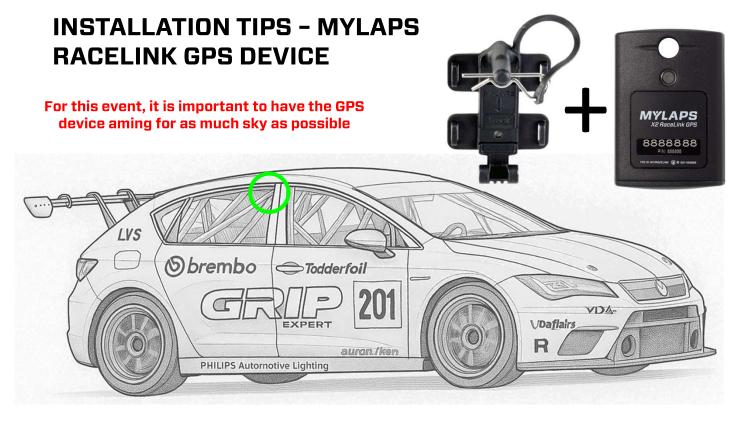
▲ **Best suggestion**: Fit the wireless *Racelink GPS* on the safety roll cage at near the top of the window or roof of the car. Aim for as much "vision" from the RaceLink GPS to the sky.
