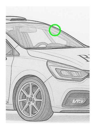
▲ **Alternative**: *Racelink GPS* positioned on the rear wing connection arms or near the roll cage bar at the front window.
